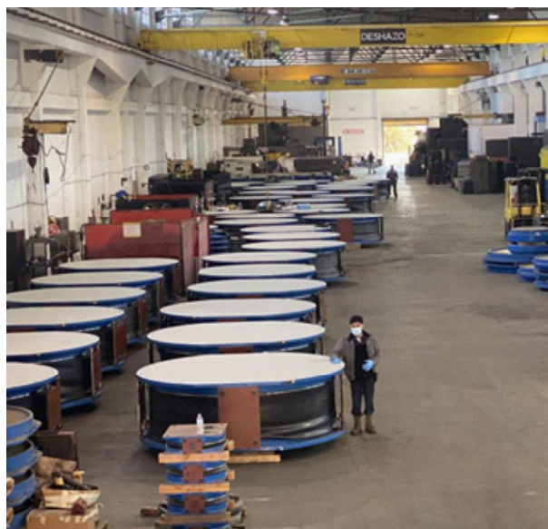
Figure 8: Isolation bearings at EPS' factory (left) and during installation on site (right).
