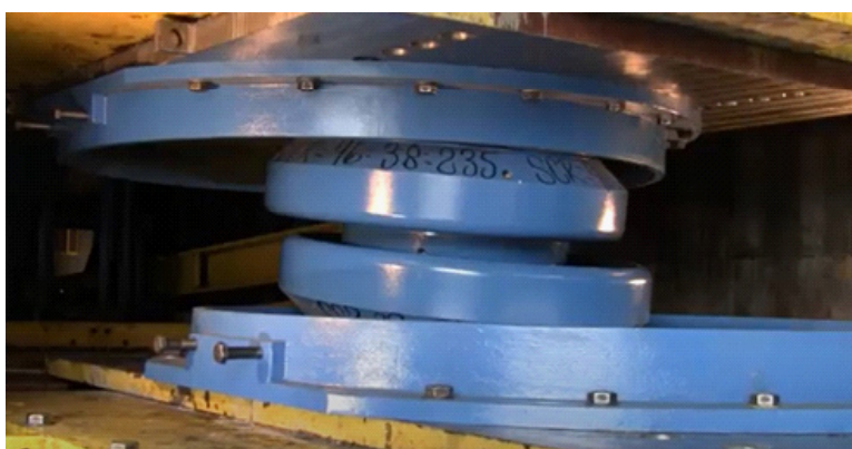
Figure 7: Prototype testing of one of the bearings at EPS (full-scale).
